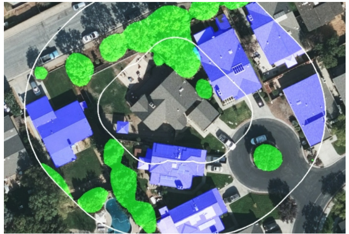
Blue represents buildings and green represents trees within 30 foot and 100 foot zones of defensible space.
