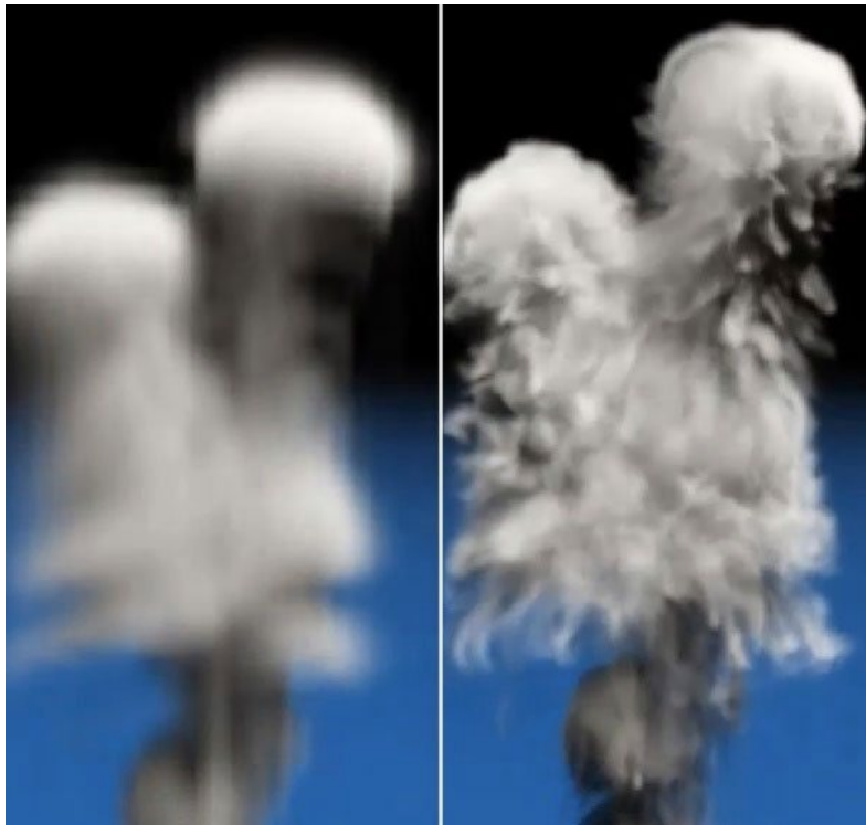
Figure 10. Interpolated physical model output of a smoke plume (left); a fine scale component of the flow is added by physically constrained ML algorithms to create realistic high-resolution model output (right). (Source: CS, Cornell University)
